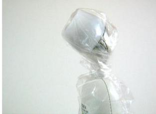
1. Insert sensor head end first and twist sheath at neck with fingers to assure film is smooth over sensor head lens.
