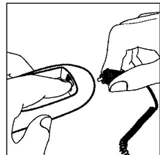
4. Replace the battery into the compartment. Re-install battery cover.
