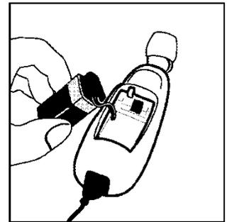
2. Depress black release button and remove cable while holding the release button down.
