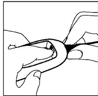
3. Orient cable plug properly for proper fit into the receptacle hole and install replacement cable.
