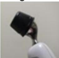
Apply cap by pushing onto the probe head with fingers. After temperature measurement is completed, remove the cap by pushing edge forward with thumb. (Figure 2)
