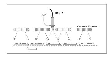
below 200°F (93°C) and to keep the lens clean. The IRt/c.3x is the preferred model for this application because of its small physical size and built-in air purge. It can function in temperatures to 250°F (121°C) when the air purge system is used. For still narrower fields of view, the IRt/c.5 and IRt/c.10 with 5:1 and 10:1 FOV respectively are very popular.
