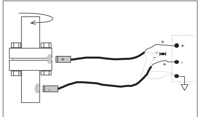
(connecting the two minus leads together and measuring across the plus leads, see example), measuring the difference in temperature between the joint and adjoining shaft. This difference is a direct measure of the heat created in the joint and will not be influenced by ambient temperature effects, since the differential pair arrangement cancels those effects. Accordingly, a very high precision can be achieved. An IRt/c with built-in air purge is recommended if the environment is oily or dusty.
