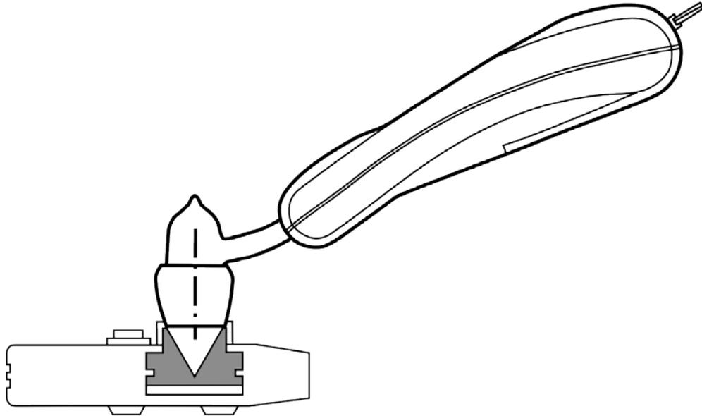
7. **Compare CM Reference Thermometer readings to test thermometer.** Refer to instruction manual for particular model being verified. Alternately insert the CM thermometer and the thermometer being verified into the portable blackbody calibration verifier opening, comparing readings to the CM.
