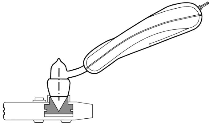
**Figure 1. Portable black body is used to verify the calibration of any TAT-5000 or TAT-5000S vs. a Certified Master, by comparison of readings.**
