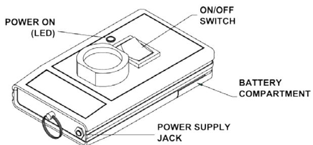
**Figure 2. Model PBB-1 Portable Blackbody Calibration Verifier**
