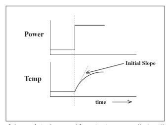
If the IRt/c is clean and functioning normally, it will report the correct rate of change, and the machine becomes operational. If the rate of change is lower than normal, the user is alerted to clean the lens. If this still does not produce the desired response, service is required on the IRt/c or heater, target, control, etc.
