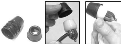
1. Apply cap by pushing onto the probehead with fingers.
