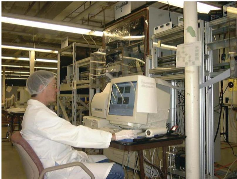
Exergen's stringent calibration techniques subject each product to a wide range of target and ambient temperatures, right on the factory floor, and all under precise computer control. This advanced calibration system ensures the best accuracy available in the industry, meeting all relevant standards. For our own record keeping and unit traceability, every product is programmed with a unique serial number, and all calibration records are kept in a database. Our process is TUV and UL approved.
