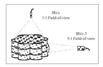
monitor specific areas from greater distances. Actual fire types and special conditions should be evaluated prior to applying IRt/c's.
