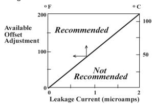
accurately, but the temperature indication will be incorrect. Accordingly, recommended controllers are those which have low leakage currents and/ or sufficient offset adjustment to produce an accurate IRt/c reading (see chart for relationship between leakage current and offset).
