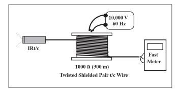
module to a computer. As a noise generator, a 60 Hz 10,000 volt transformer and spark generator was set up to spark within 6 inches (15 cm) of the wire. The test results showed less than 0.1°C of noise at any relative position of the wire, spark, and transformer.
