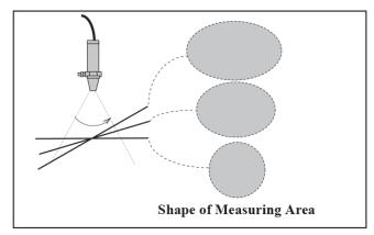
To apply this method, be sure to estimate the size of the field-of-view footprint, and confirm that the IRt/c is measuring the area you wish to measure.
