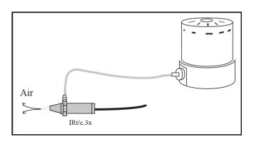
only a few minutes to install; and its small size; Air Pump Kits provide you a convenient and inexpensive assurance of long term, trouble-free operation of your IRt/c temperature control system.
