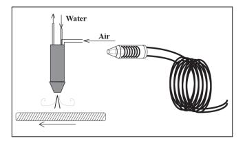
The water cooling system consists of a seamless monotube, in order to eliminate the possibility of leaking joints. For convenience, the seamless tubing includes an extra 3 ft (1 m) tubing length.
