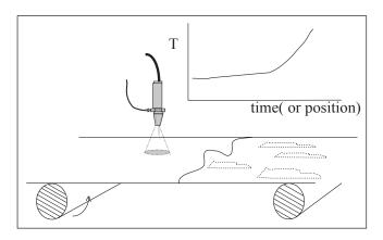
A simple implementation method is to measure the difference in temperature between the product and the ambient air. Determine the delta T that results in the correct dryness, and set the control system to maintain that delta T.
