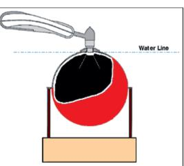
An inexpensive certified-emissivity blackbody offers accuracy and traceability to recognized standards and mathematics.
