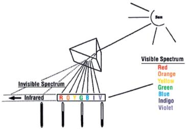
Figure 1. Herschel's experiment demonstrated that heat is generated beyond the visible spectrum.
