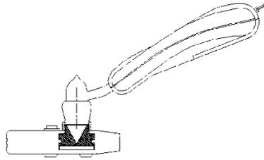
Using a Certified Master Reference Thermometer in a Portable Blackbody to Verify Calibration
