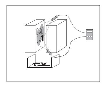
connected to a single controller, so that a part viewed by either sensor will alarm.
