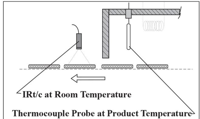
Mechanical changes occur because conventional thermocouples are generally constructed as small and light as possible to enhance response time, making them vulnerable to deformations that can change the thermoelectric properties. More importantly the conventional thermocouple must operate at elevated temperature since it merely measures its own temperature.
