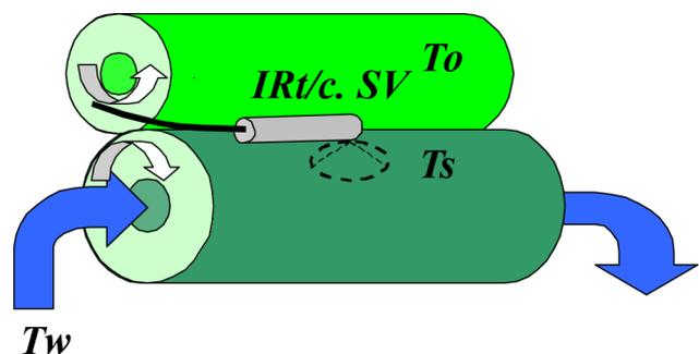
Figure 2. Cooling roll controlled by IRt/c sensing inked surface temperature.
