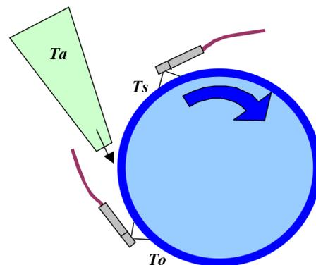
Figure 6. Air-cooled arrangement showing two IRt/c's monitoring the roll surface temperature just prior to the air jet ( $T_o$ ) and just after the air ( $T_s$ ). The air supply temperature ( $T_a$ ) can be monitored with a standard thermocouple.
